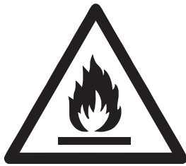
caution, risk of fire
